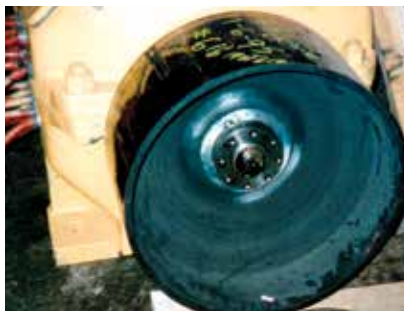
Superbolt mill motor nuts are special jamnuts designed to fasten brake wheels, couplings, and pulleys to mill motors. They are directly interchangeable with nuts supplied by the motor manufacturers.
